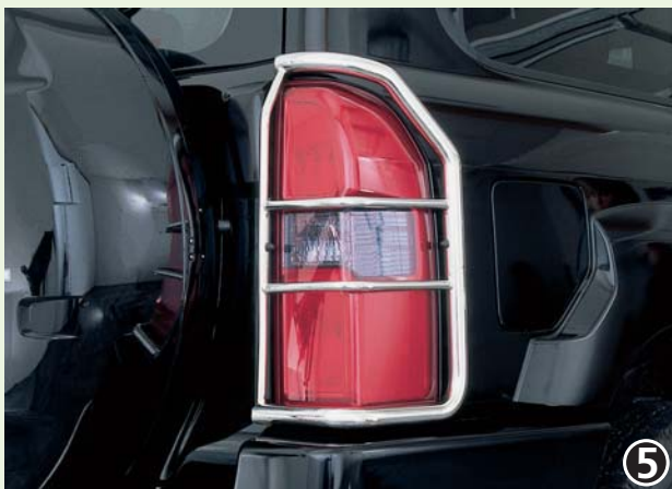
Rear pipe frame 28mm single pipe with lamp grill (5-door) Heckrohrrahmen 28mm mit Lampenschutzgitter (5-Türer) Stainless steel/Edelstahl
