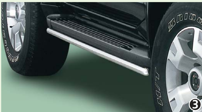
Side step protection pipe 42mm (5-door) Trittbrettschutzrohr 42mm (5-Türer) Stainless steel/ Edelstahl
